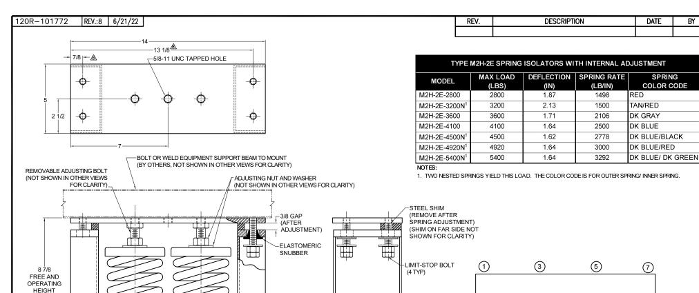
1/4 RIBBED **ELASTOMERIC** PAD (2 TYP) 5/8 DIA HOLE (4 TYP)
